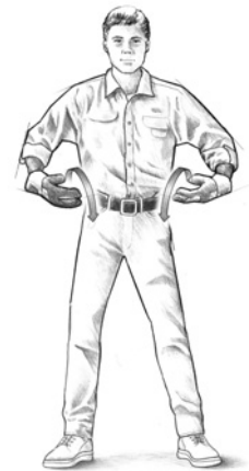
7) Drive assist Tells driver to give the tires more drive force to assist the winching process.
