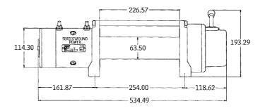
534mm L. x 160mm D. x 193mm H. Mounting Bolt Pattern: 254mm x 114.3mm
