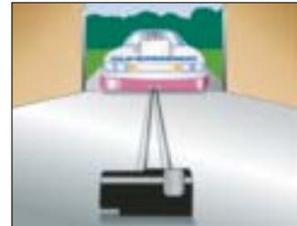
Right angle pull with pulley block    Double line pull with pulley block
