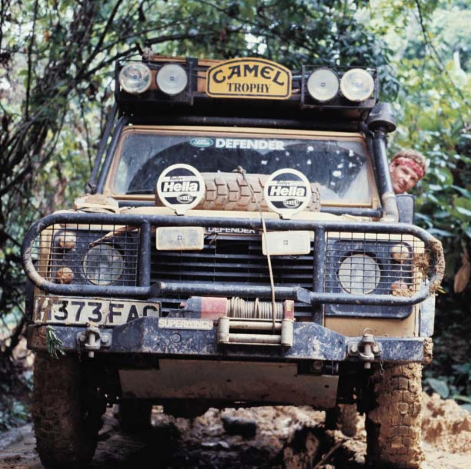
**The Superwinch Husky Series – we dare you to find tougher winches. With their rugged worm-gear drive mechanism and 4.2 horsepower series wound motors, the Husky 8 and Husky 10 are two off-road champions in their own right. The case-hardened nickel spur gears and steel-centered phosphor bronze wormwheel matched to a case-hardened ground and polished worm shaft make this winch virtually indestructible. When only the best will do – the only choice is a Superwinch Husky.**
