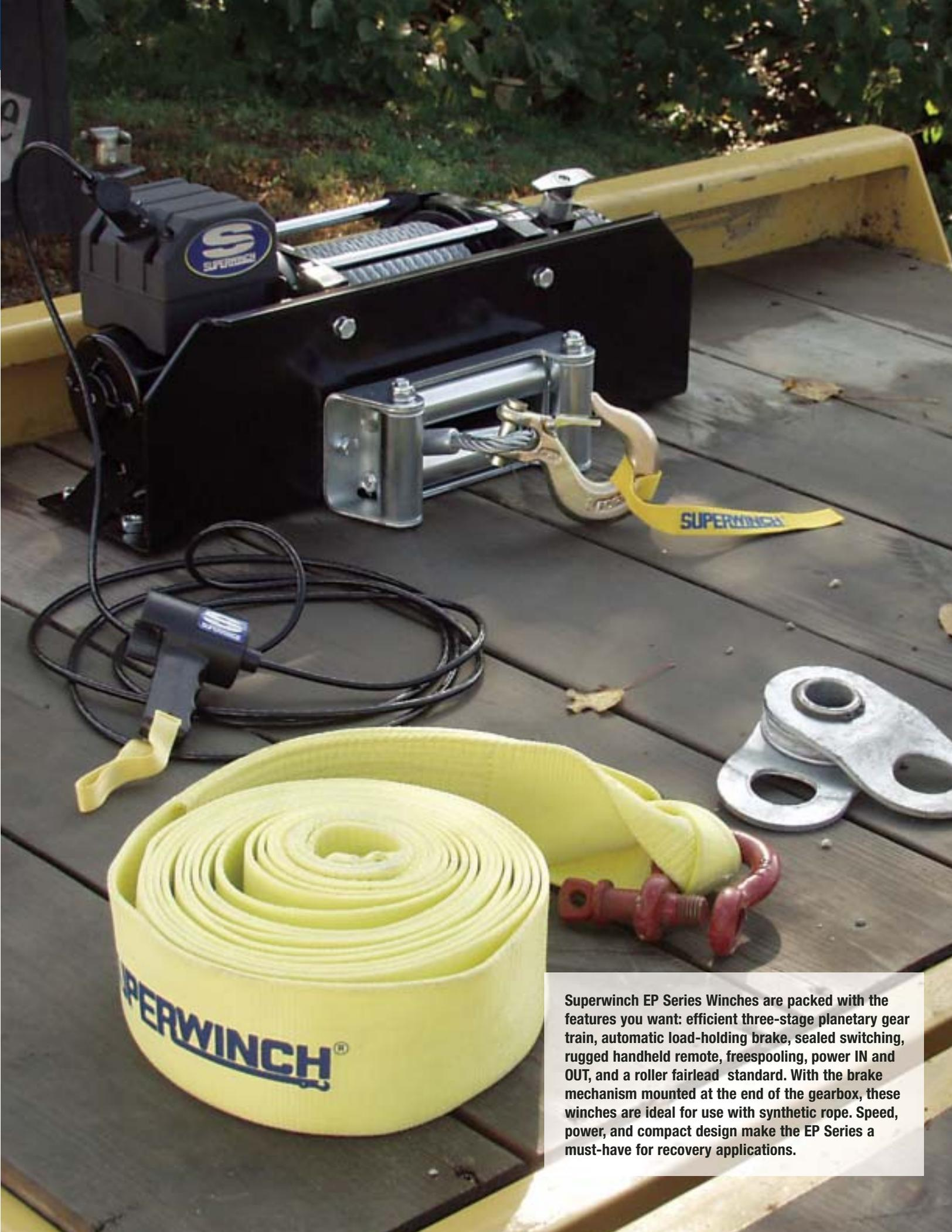
Superwinch EP Series Winches are packed with the features you want: efficient three-stage planetary gear train, automatic load-holding brake, sealed switching, rugged handheld remote, freespooling, power IN and OUT, and a roller fairlead standard. With the brake mechanism mounted at the end of the gearbox, these winches are ideal for use with synthetic rope. Speed, power, and compact design make the EP Series a must-have for recovery applications.
